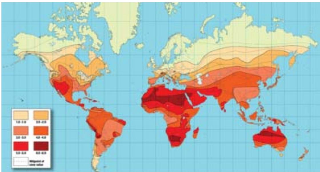
Figure A-4 Worldwide average solar irradiation (kWh/m<sup>2</sup> per day)
