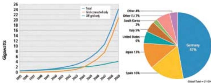
Figure A-5 Solar PV: Existing world capacity 1995 to 2009 (left) and top six countries by cumulative capacity 2009 (right) (REN21, 2010)
