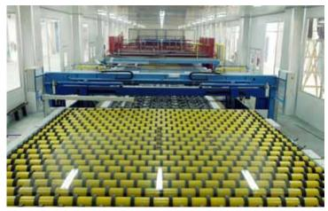
Functions and use: This technology is mainly used on 500-1,200ton-level large float glass production lines. It reduces energy consumption in glass production, accurately controls process parameters for big tonnage glass production lines and stabilizes glass quality.
