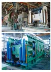
Functions and use: Rolling Press adopts the principle of high pressure material layer smashing. It squeezes materials which enter the squeeze zone and thus smashes materials and improves their grindability. Rolling presses are widely used in the breaking
