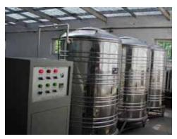
block structure, the equipment features a small footprint, offers greater flexibility than civil construction, is easy to install and use. The whole set of equipment adopts automatic control, lowpower consumption design, can run automatically according to the water volume and shut down automatically when there is no wastewater.
